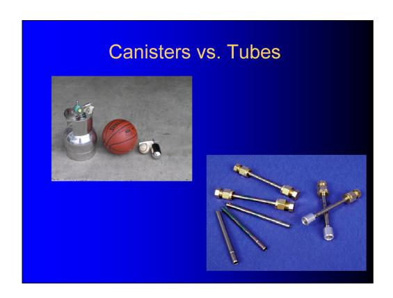
New style adsorbent tubes are much smaller than bulky canisters and can't be broken.
