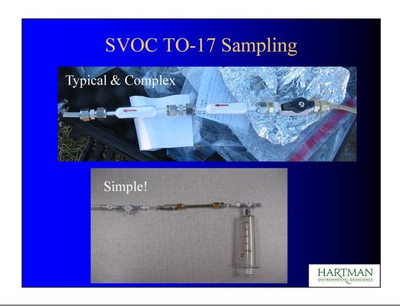
Top photo: A typical sampling arrangement used for collection of samples on adsorbants. Note the abundance of fittings and the need for duplicate cartridges for breakthrough. A very complicated set-up, prone to leaks.
